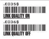
Link Quality (activated by default) ensures a more secure data transmission from the scanner to the cradle/host. To accelerate the transmission speed, you may disable Link Quality, but the data transmission integrity might become less reliable.
