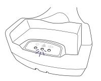
The blue LED indicator on the cradle will turn on to verify a successful connection to the scanner.
